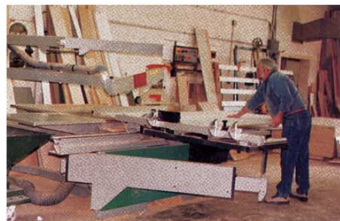
Pre-laminated boards are cut to size on an Altendorf F-45 panel saw.
